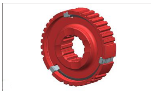
d. Assemble spring lock ring in synchro hub and lock the all strut on both side .
