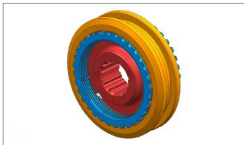
g. Assemble the synchro cone on both side.
