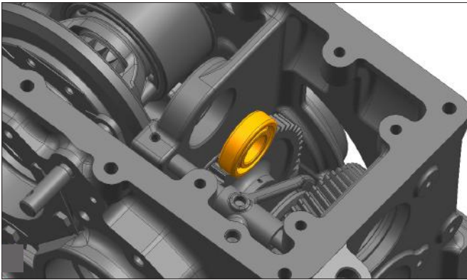
51. Assemble ball bearing 6205 in transmission housing by using mandrel 18ME244.
