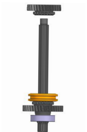
e. Insert the 3RD dog gear.
