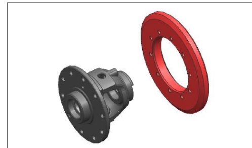
h.Remove the crown wheel.
