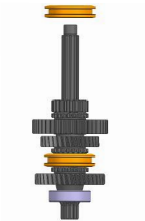
i. Insert the shifter sleeve.
