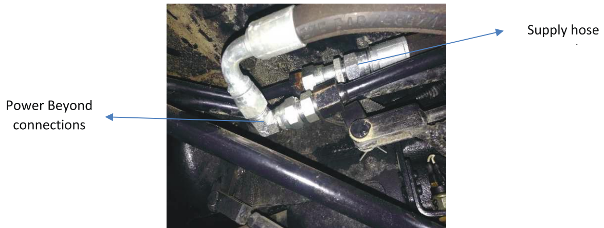
SOLIS 24 PB and SUPPLY connections (below left side platform of tractor)
