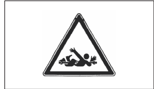
Fig. 4.12d: Warning: Do not open or remove safety shield when engine is running.
